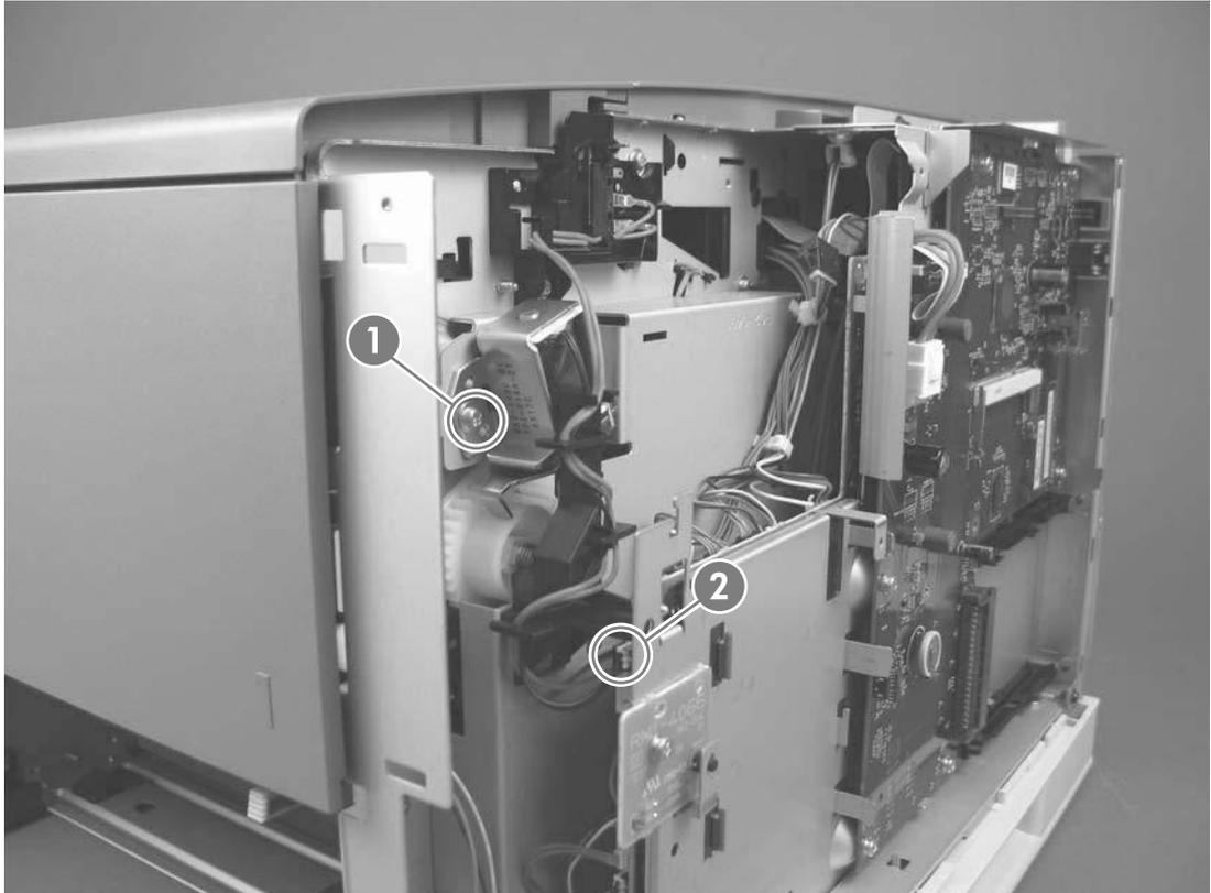
Figure 5-44 Removing the tray 1 solenoid
