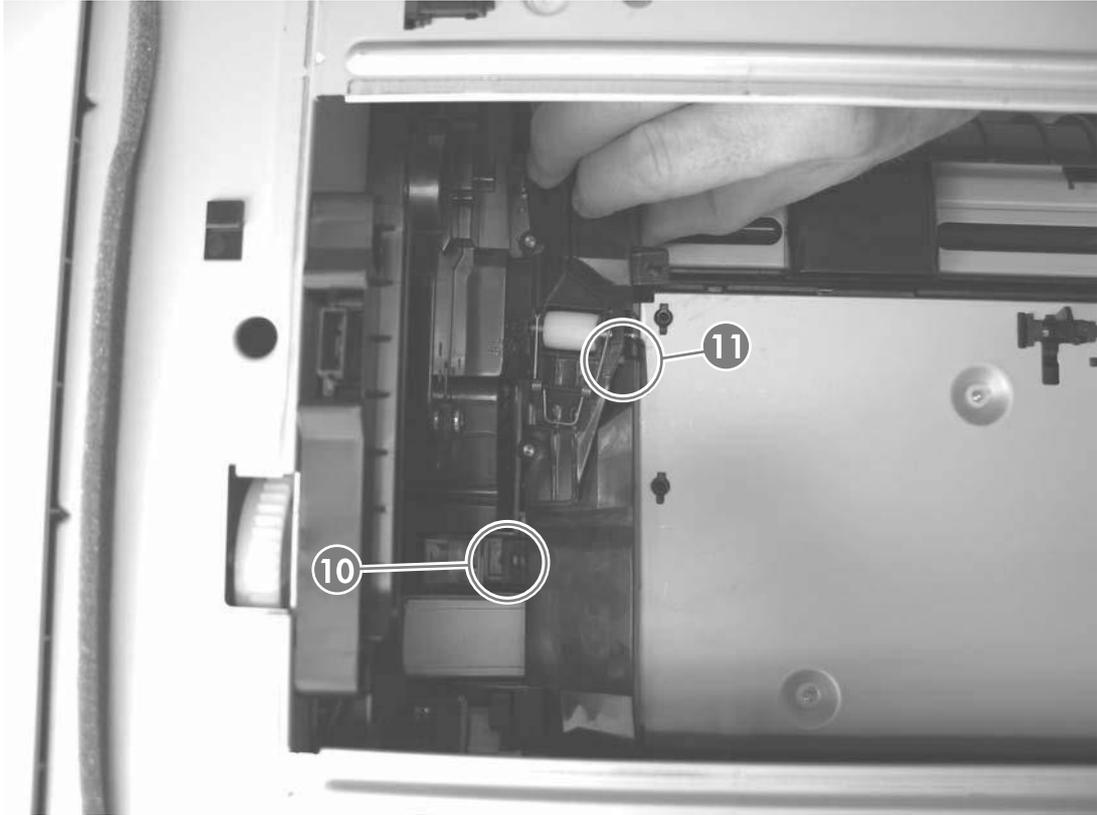
Figure 5-37 Reinstalling the oblique-roller assembly
