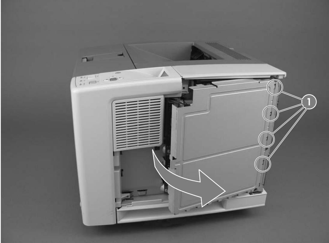
Figure 5-13 Removing the formatter (1 of 3)
