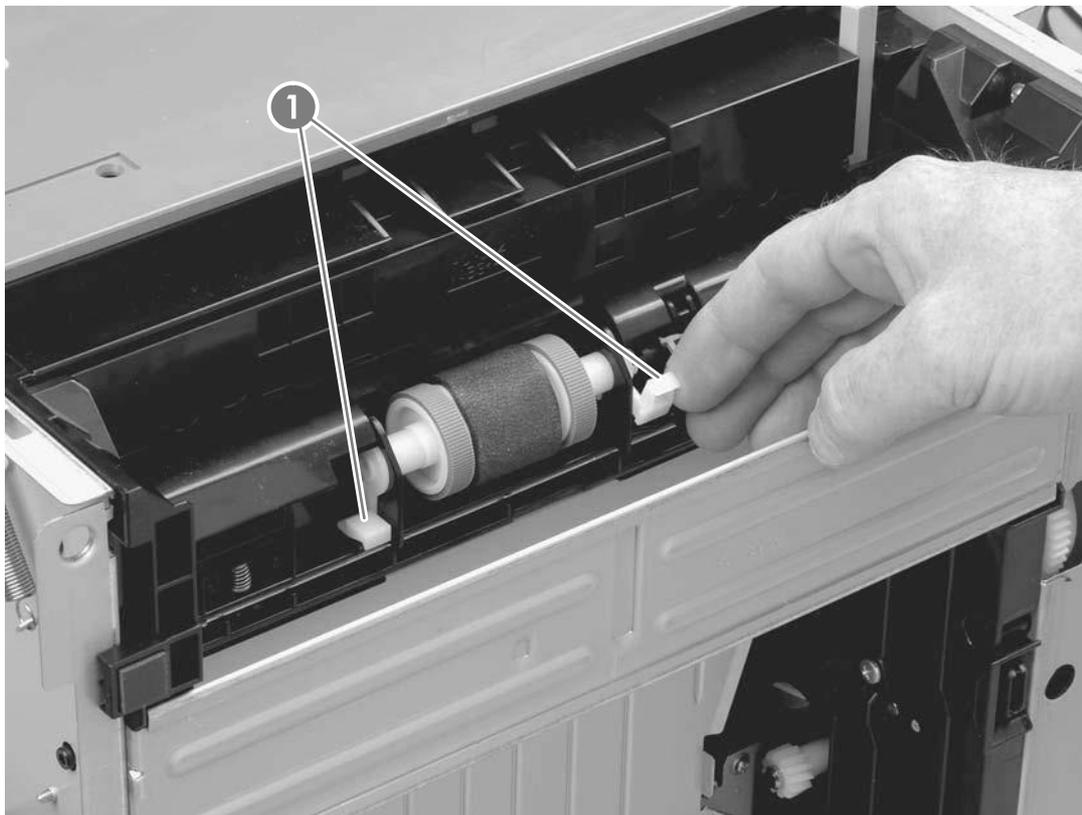
**Figure 5-58** Removing the tray 2 pickup roller (1 of 2)
