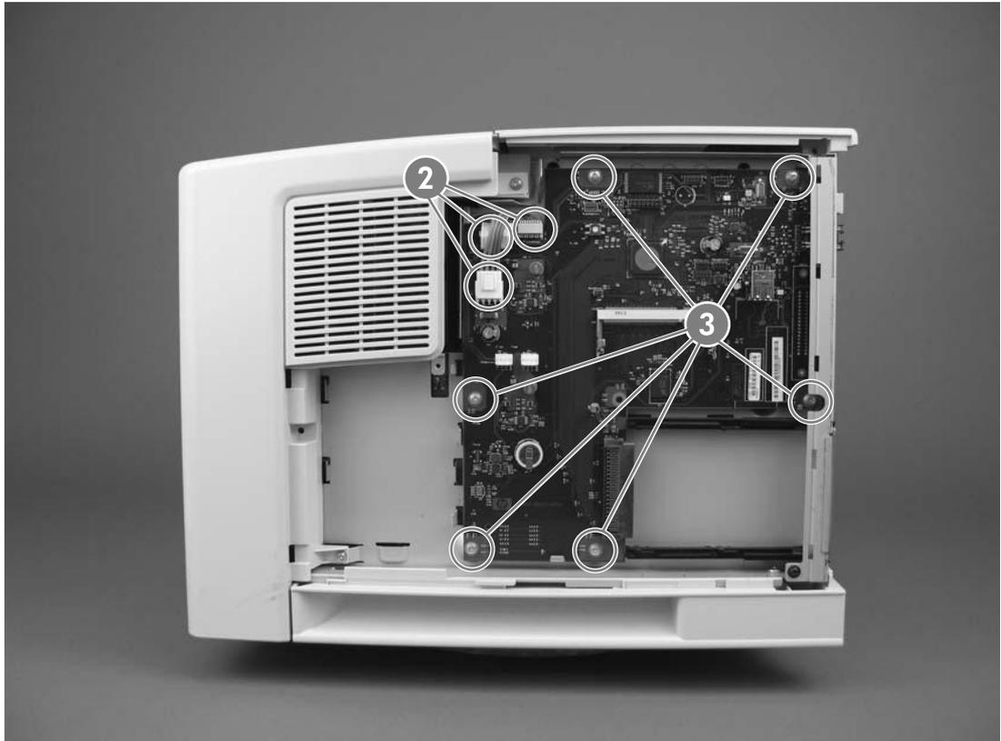
Figure 5-14 Removing the formatter (2 of 3)
