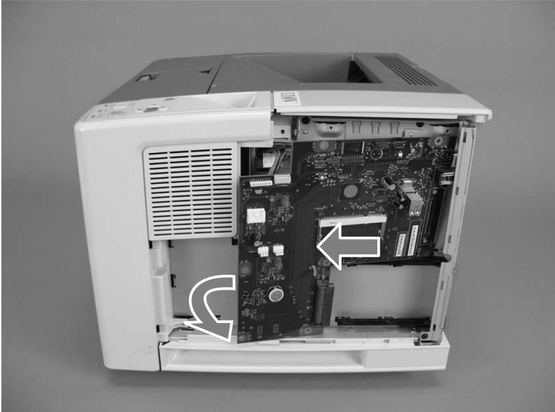
Figure 5-15 Removing the formatter (3 of 3)
