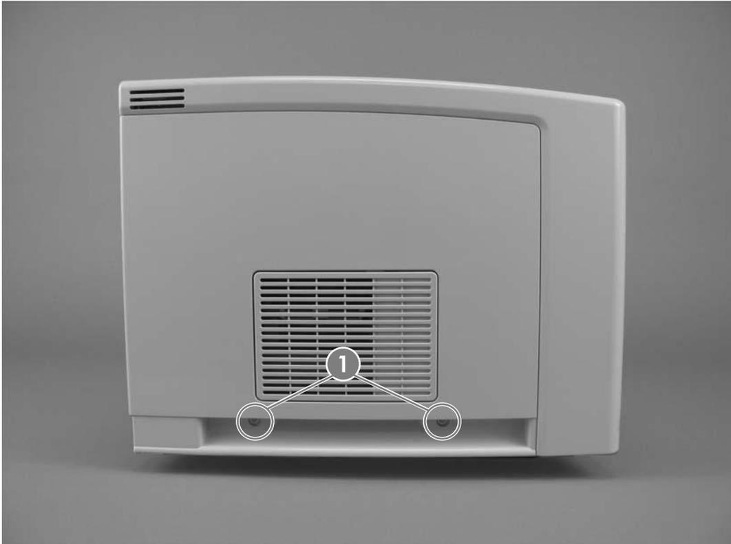
Figure 5-3 Removing the left-side cover (1 of 2)
