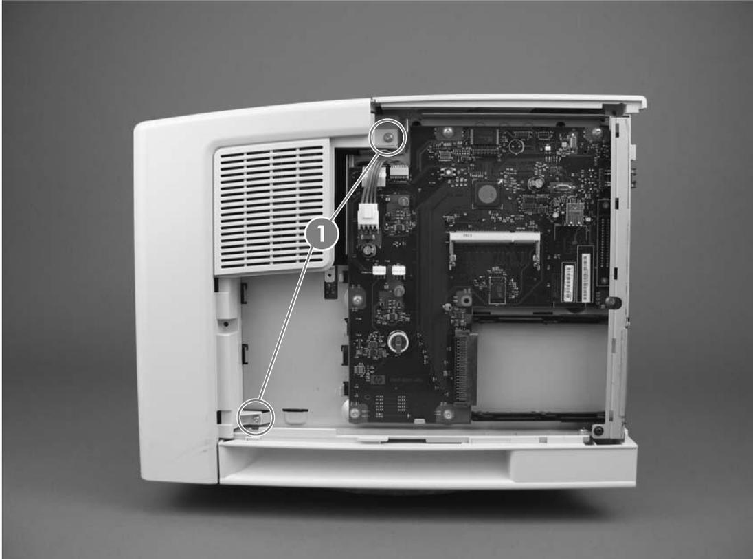
Figure 5-9 Removing the front, right cover (1 of 2)
