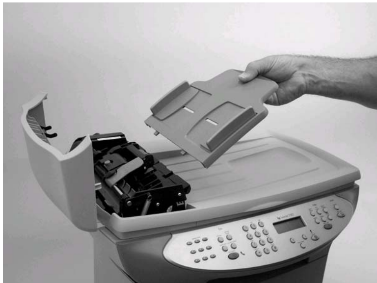
Figure 5-12. Remove the ADF pickup-roller assembly (1 of 5)
