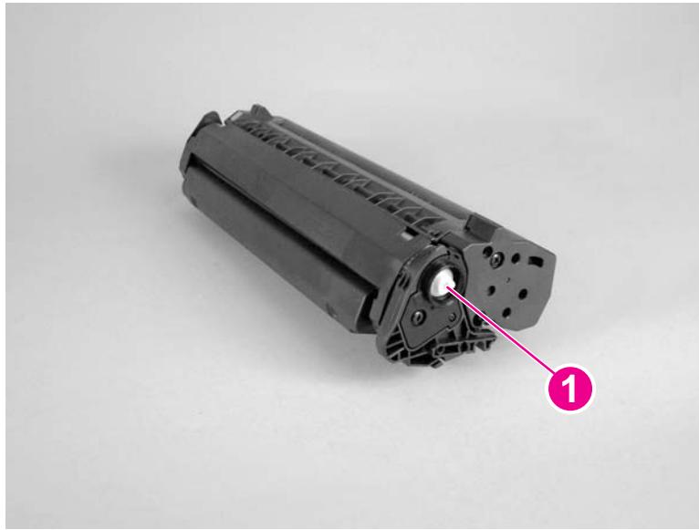
Figure 6-4. Print cartridge high-voltage connection points (right side)
