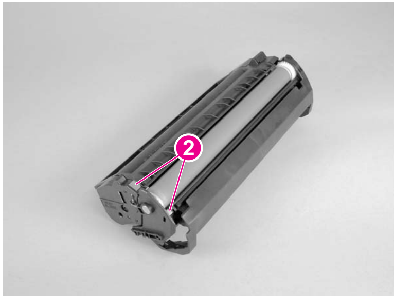
Figure 6-5. Print cartridge high-voltage connection points (left side)
