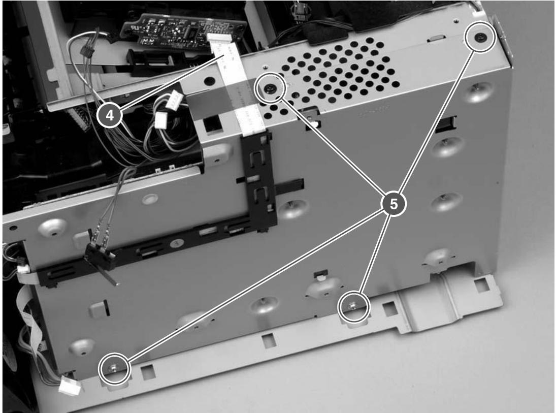
Figure 6-31 Removing the ECU (3 of 6)
