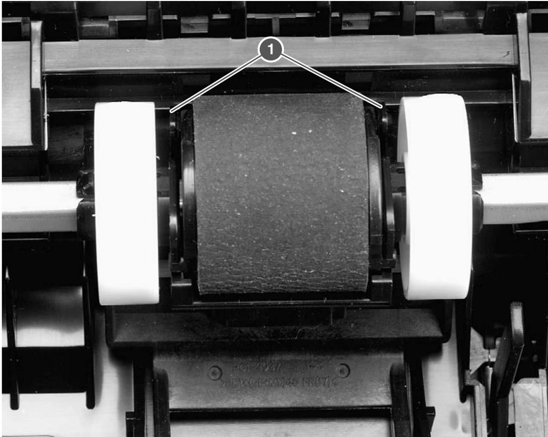
Figure 6-58 Removing the tray 1 pickup roller
