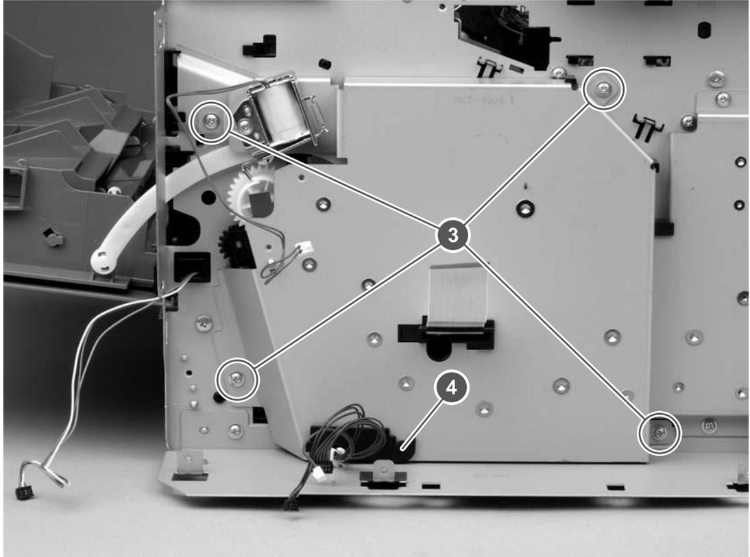
Figure 6-43 Removing the gear assembly (3 of 6)
