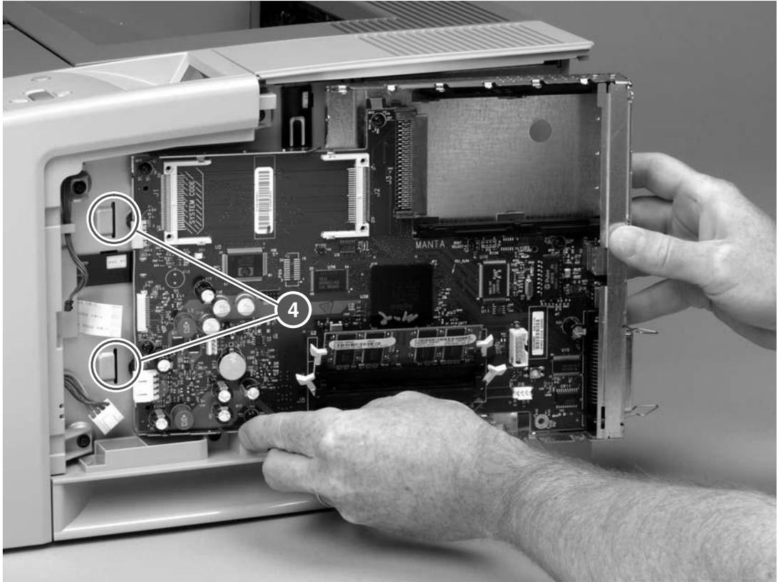
Figure 6-17 Removing the formatter (3 of 4)
