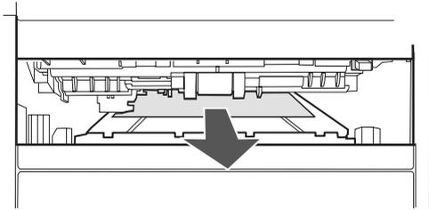
4. Push the bottom of the paper-access plate back up until it clicks into place on both sides (both sides need to be engaged).
