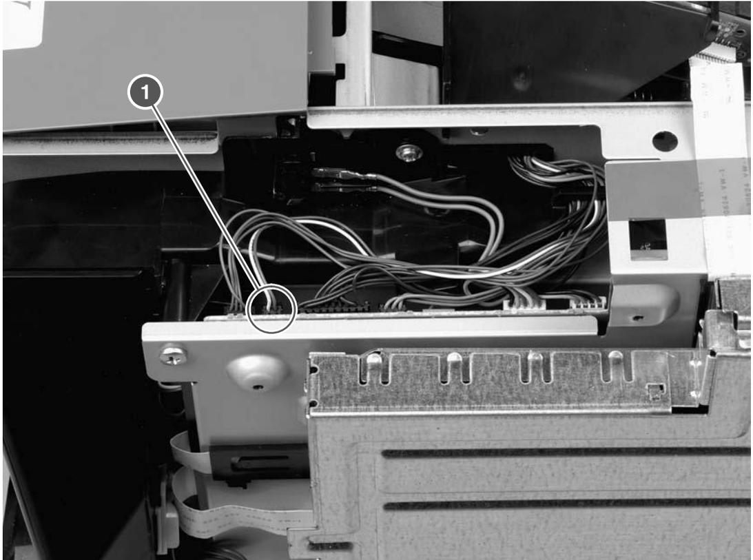
Figure 6-47 Removing the e-label reader (1 of 2)
