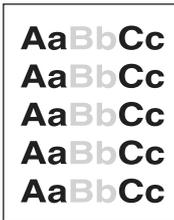
1. Make sure that the print cartridge is fully installed.
