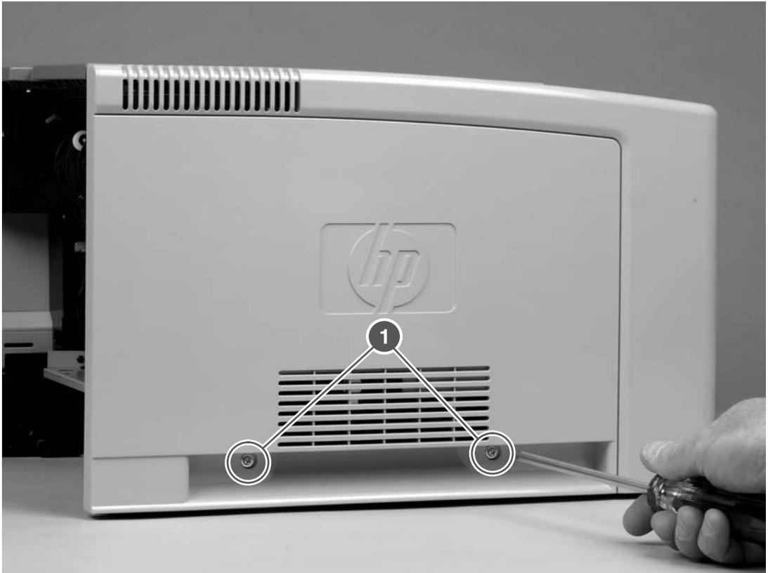
Figure 6-7 Removing the left-side cover (1 of 2)
