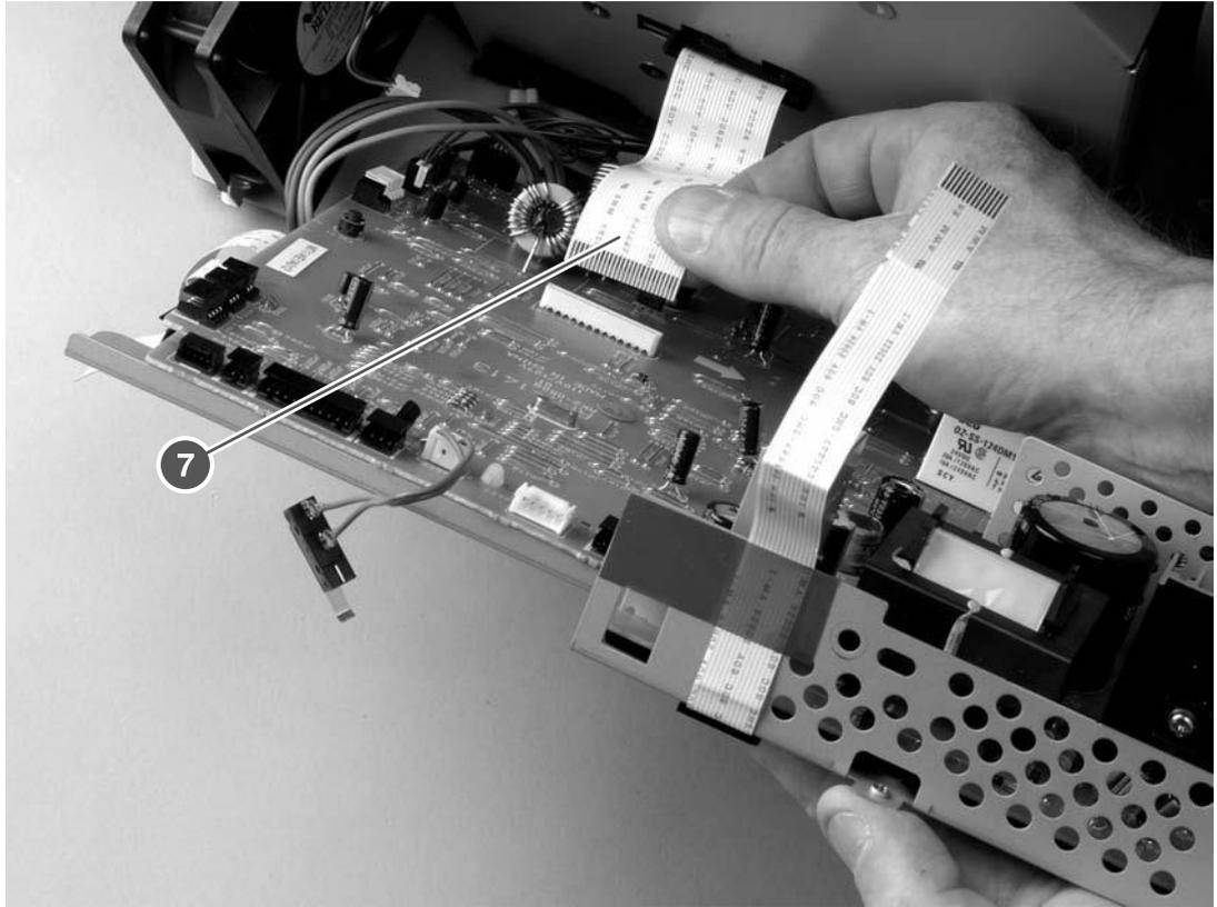
Figure 6-33 Removing the ECU (5 of 6)
