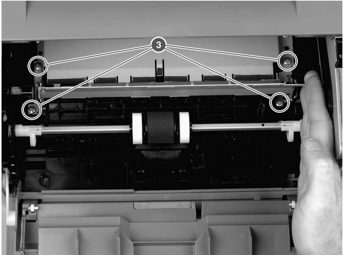
Figure 6-57 Removing the registration assembly (3 of 3)
