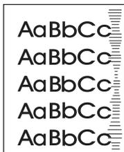
This defect typically occurs when the print cartridge has far exceeded its rated life of 6,000 (Q6511A) or 12,000 (Q6511X) pages. For example, if you are printing a very large quantity of pages with very little toner coverage.
