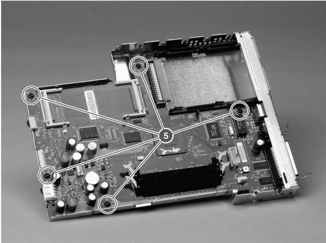
Figure 6-18 Removing the formatter (4 of 4)
