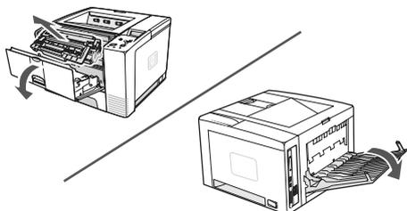
2. If the media is visible from the rear output opening, carefully use both hands to pull the leading edge out of the printer. Carefully remove the rest of the jammed media from the printer.
