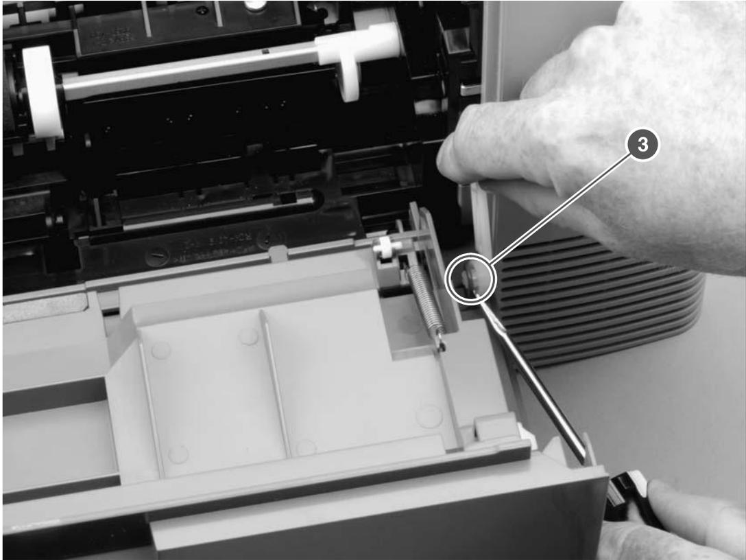
Figure 6-52 Removing the cartridge door (2 of 3)
