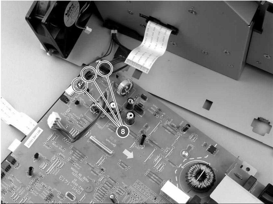
Figure 6-34 Removing the ECU (6 of 6)
