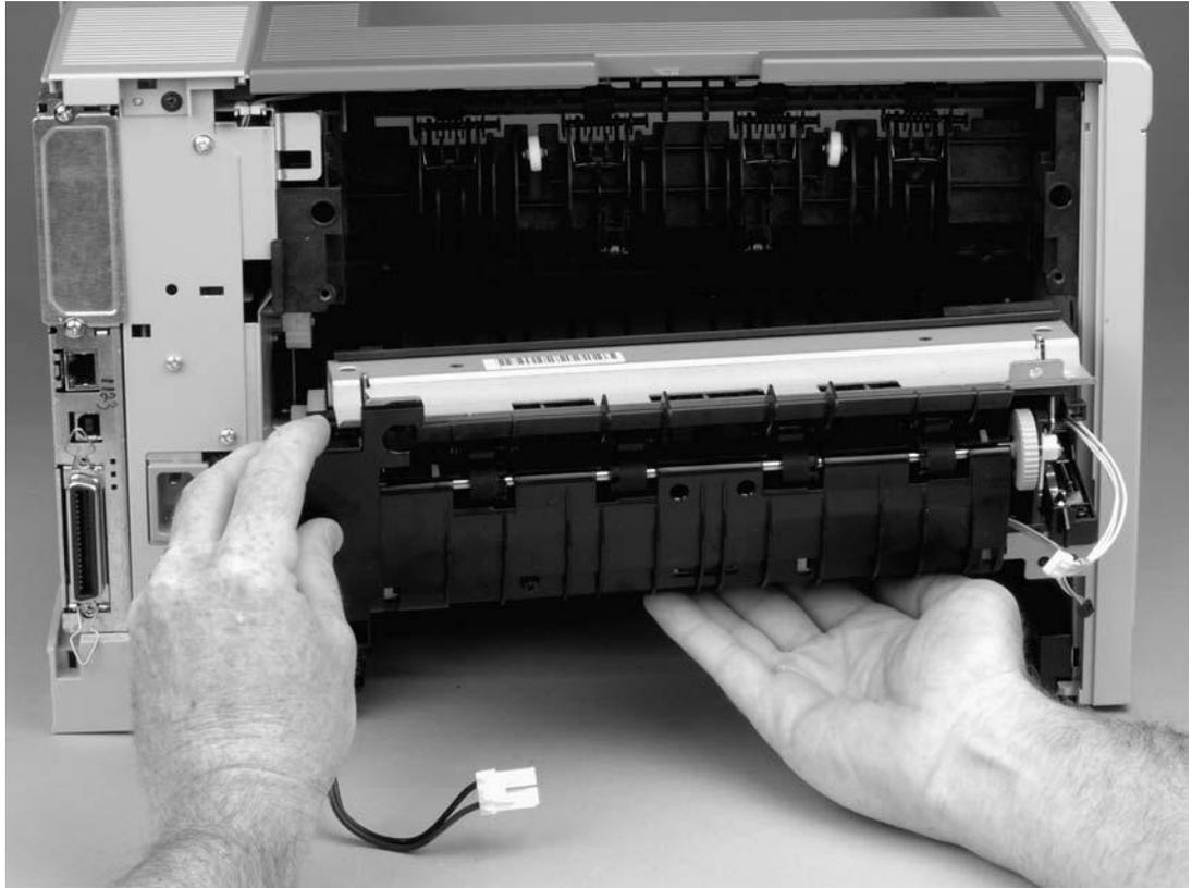
Figure 6-23 Removing the fuser (5 of 5)
