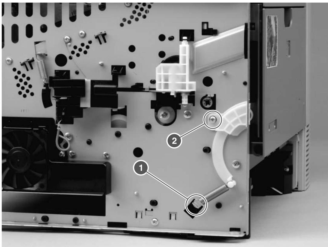
Figure 6-51 Removing the cartridge door (1 of 3)
