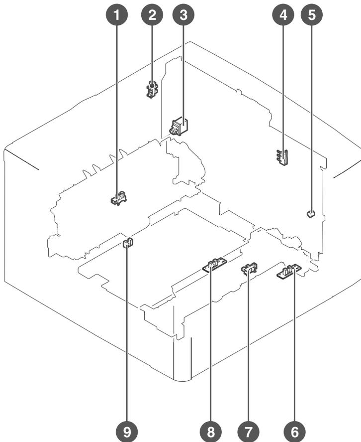
**Figure 7-8** Sensors and switches, HP LaserJet 2400 series
