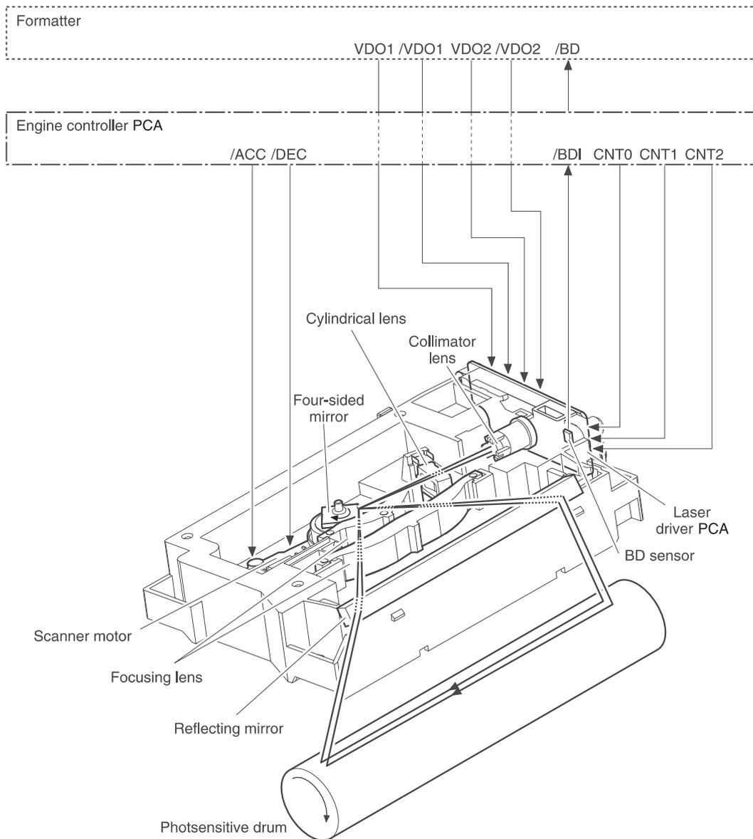
Figure 5-5 Laser/scanner system
