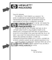
This type of defect might occur when using preprinted forms or a large quantity of narrow paper.
