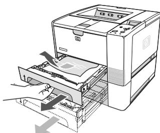
2. Remove any misfed media by pulling it out by the visible edge. Make sure that all of the media is aligned in the tray (see the user guide). If tray 3 is installed, remove any misfed media and make sure that all of the media is aligned in that tray.
