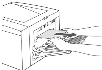
3. If the media is almost completely visible from the top output bin, pull the remaining media carefully out of the printer. If the leading edge is not visible or is barely visible in the print-cartridge area, open the rear output bin all the way. To do this, push the bin door slightly forward and use your finger to disengage the grill at the base. Turn the jam-clearing wheel to move the media out of the printer.
