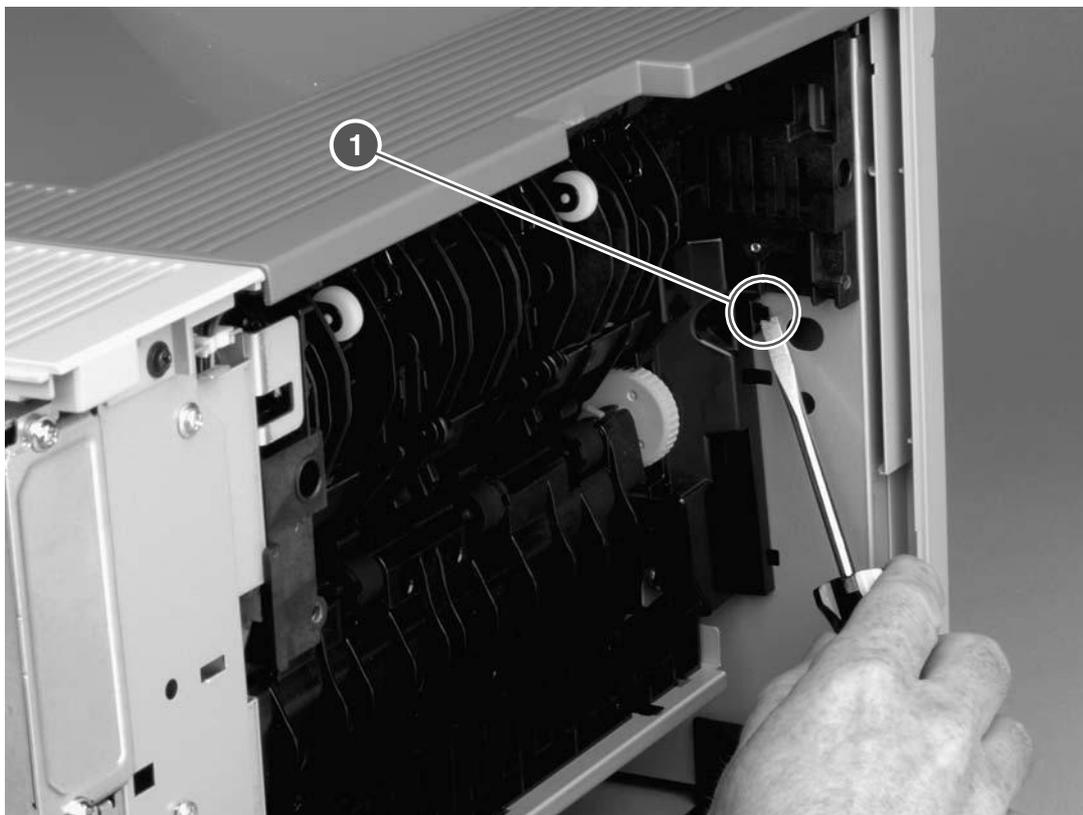
Figure 6-19 Removing the fuser (1 of 5)
