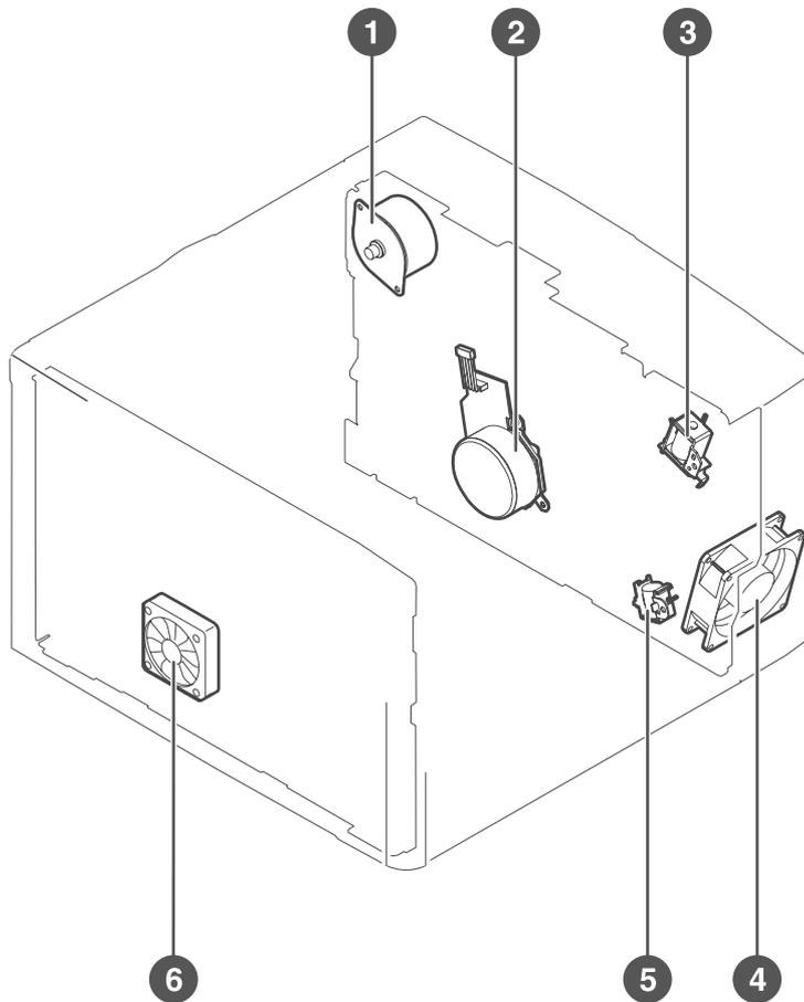
Figure 7-9 Motors, fans, and solenoids, HP LaserJet 2400 series
