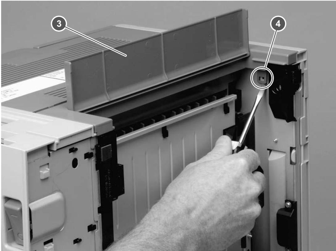
Figure 6-4 Removing the back cover (2 of 3)
