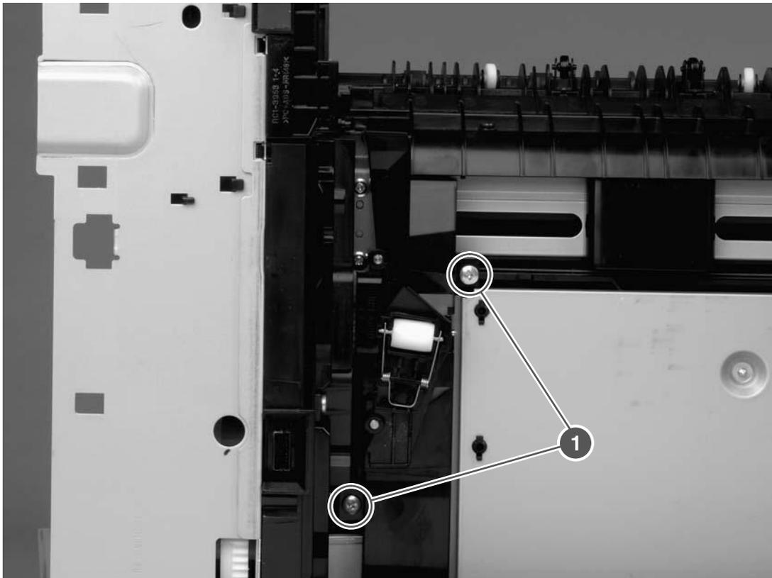
Figure 6-36 Removing the power supply (1 of 5)
