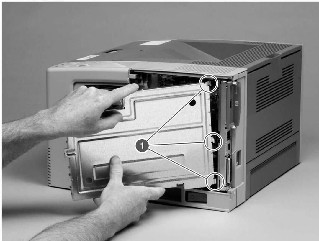
Figure 6-15 Removing the formatter (1 of 4)
