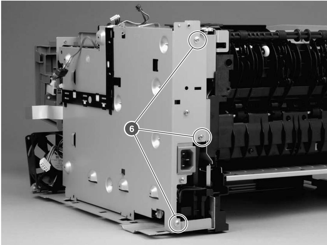
Figure 6-32 Removing the ECU (4 of 6)
