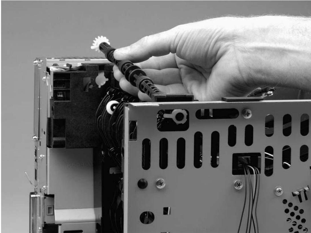
Figure 6-50 Removing the face-down-roller shaft (2 of 2)
