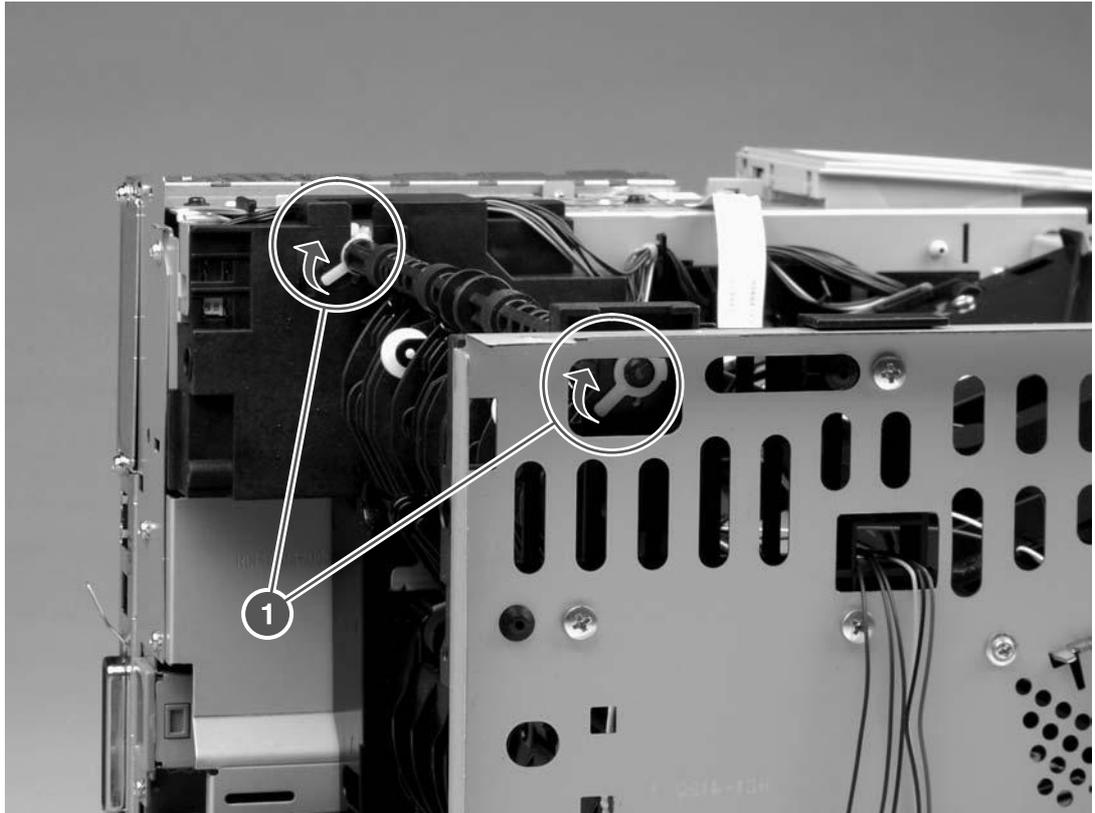
Figure 6-49 Removing the face-down-roller shaft (1 of 2)
