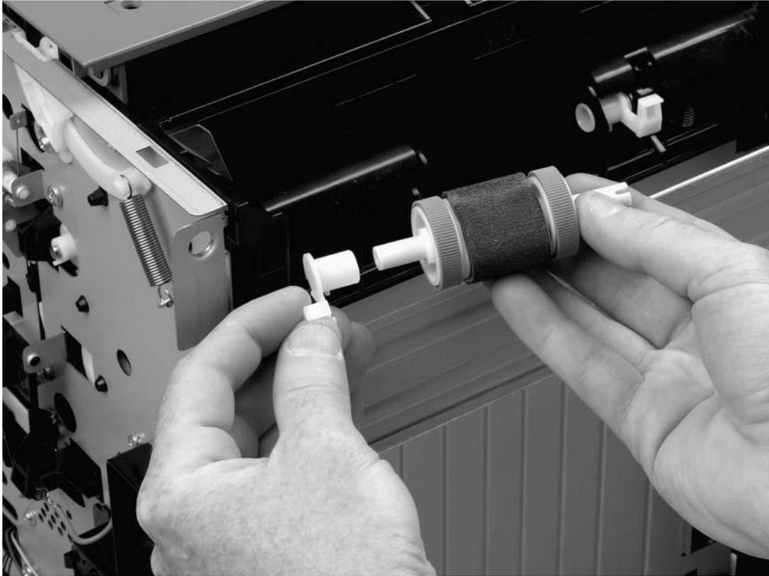
Figure 6-60 Removing the tray 2 pickup roller (2 of 2)
