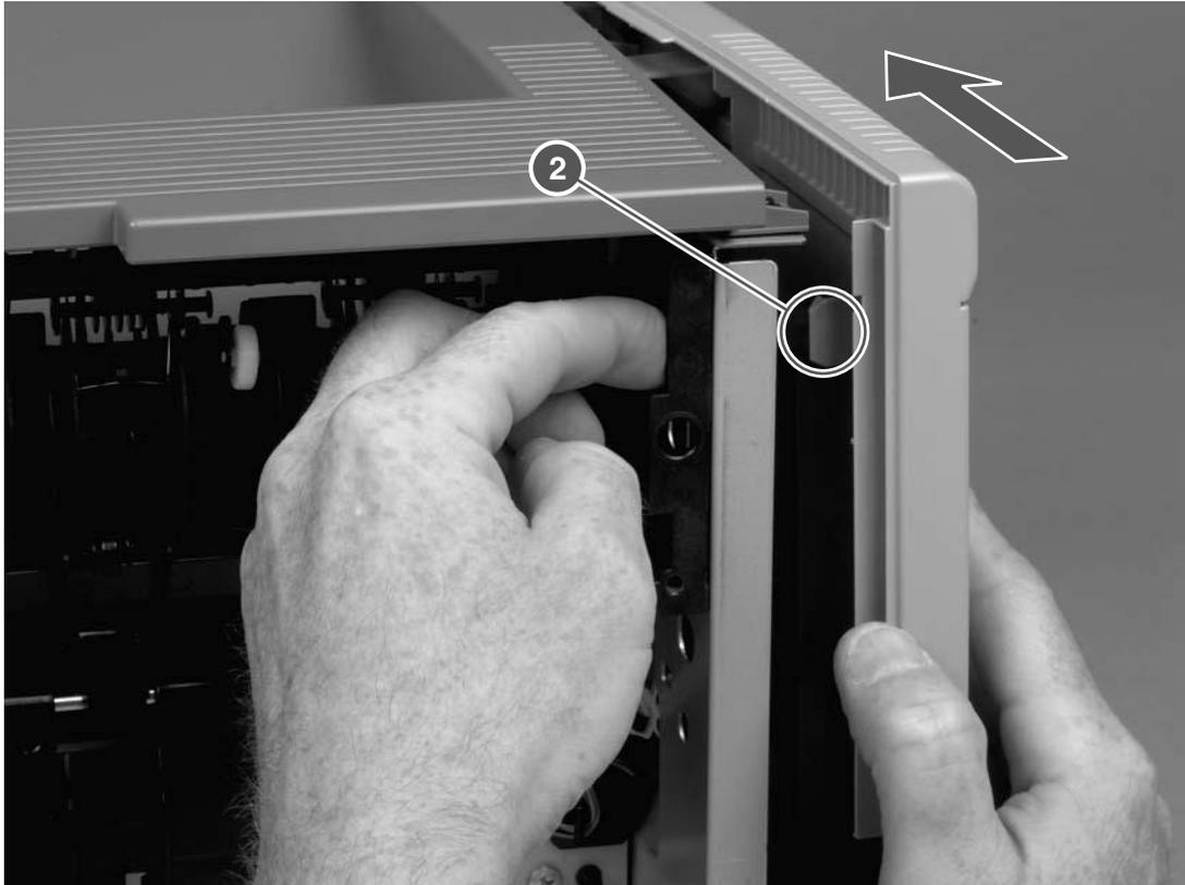
**Figure 6-8** Removing the left-side cover (2 of 2)
