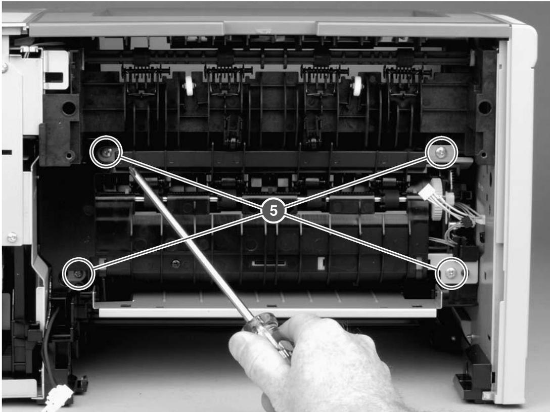
Figure 6-22 Removing the fuser (4 of 5)
