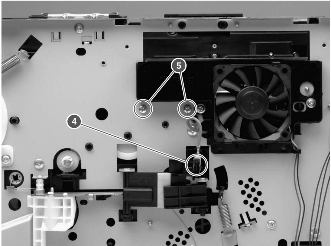
Figure 6-39 Removing the power supply (4 of 5)
