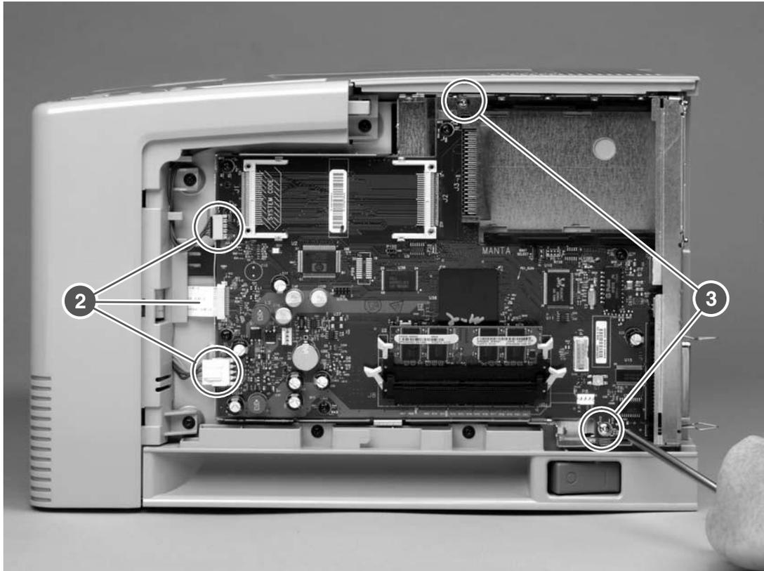
Figure 6-16 Removing the formatter (2 of 4)
