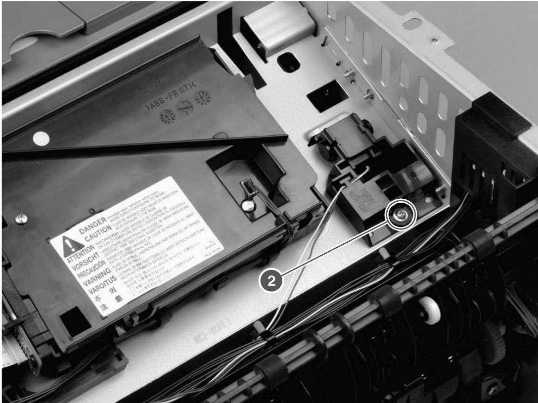
Figure 6-48 Removing the e-label reader (2 of 2)
