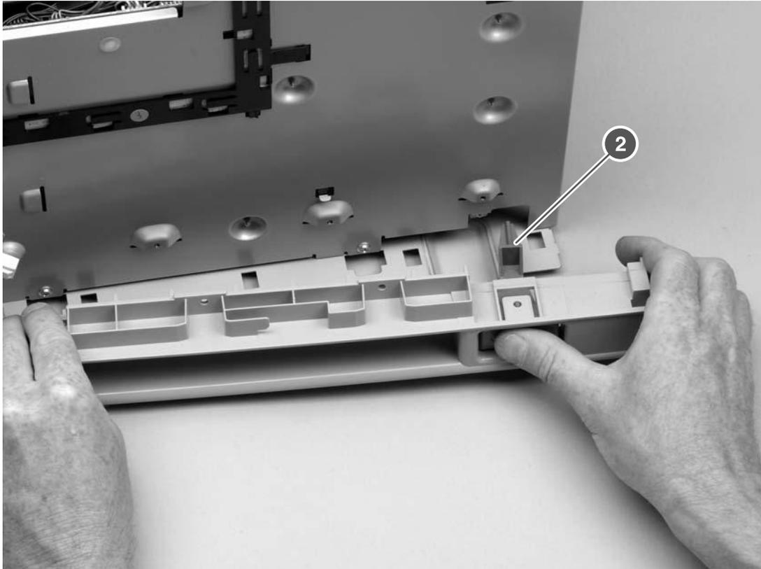
**Figure 6-28** Removing the right-side handle (2 of 2)
