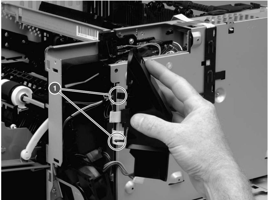
**Figure 6-29** Removing the ECU (1 of 6)
