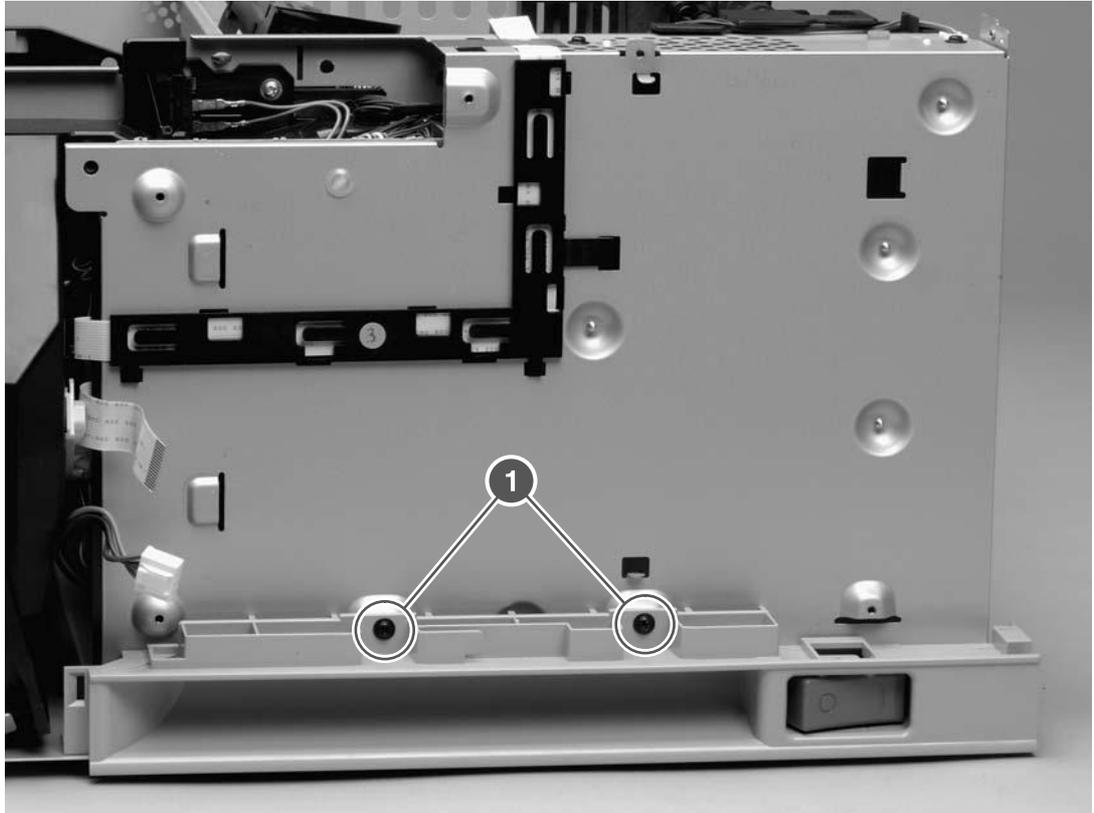
Figure 6-27 Removing the right-side handle (1 of 2)
