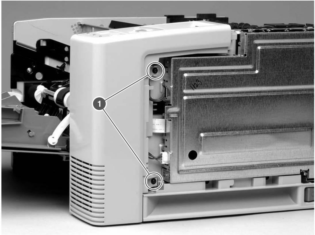
Figure 6-11 Removing the front, right cover (1 of 2)
