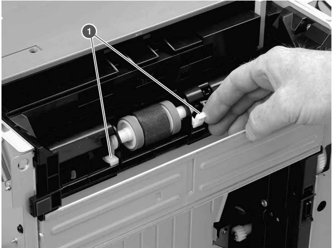
**Figure 6-59** Removing the tray 2 pickup roller (1 of 2)
