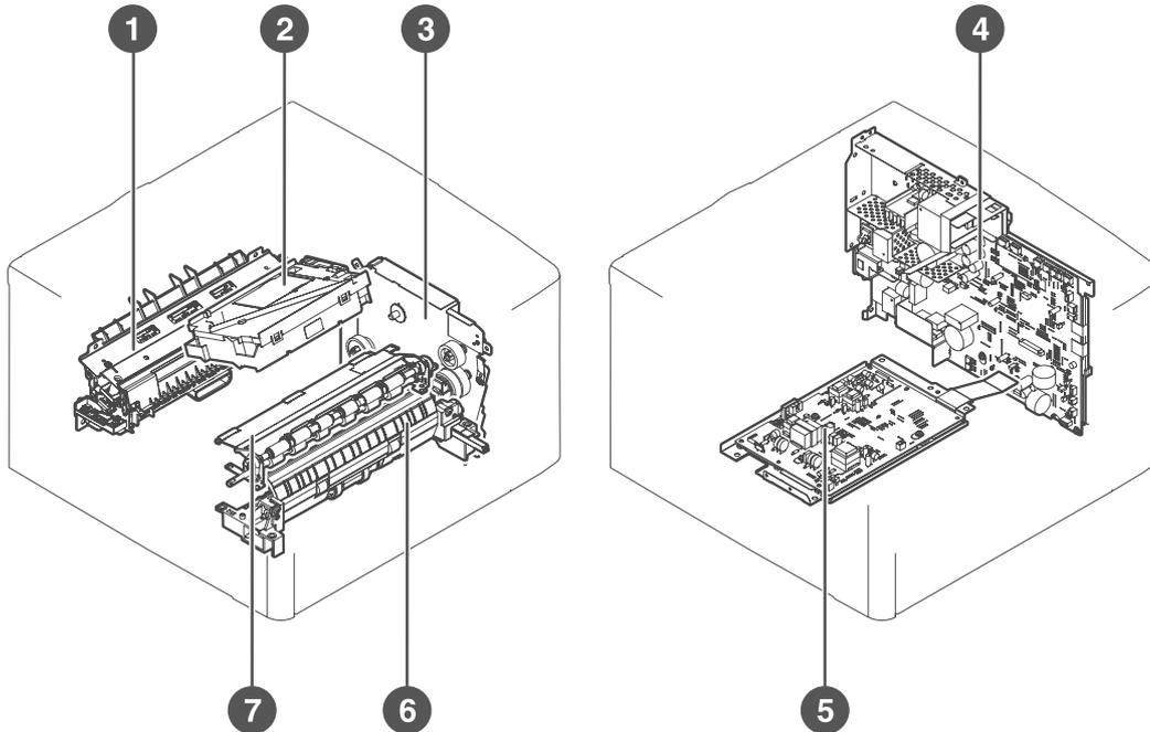
Figure 7-6 Main assemblies, HP LaserJet 2400 series
