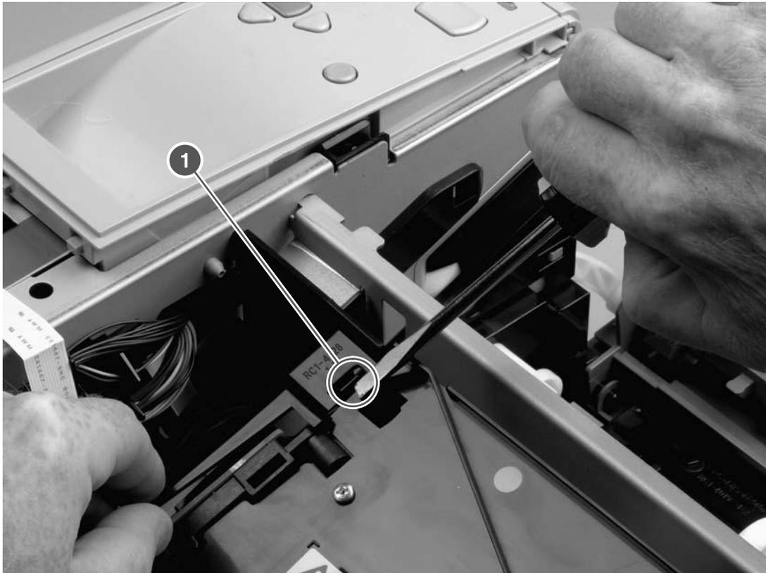
Figure 6-24 Removing the laser/scanner (1 of 3)
