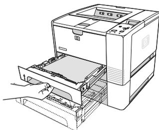
3. If the media is jammed in the paper-feed area and cannot be reached from the print-cartridge area, grasp the sheet and carefully pull it free from the printer.
