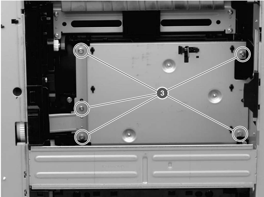
Figure 6-38 Removing the power supply (3 of 5)
