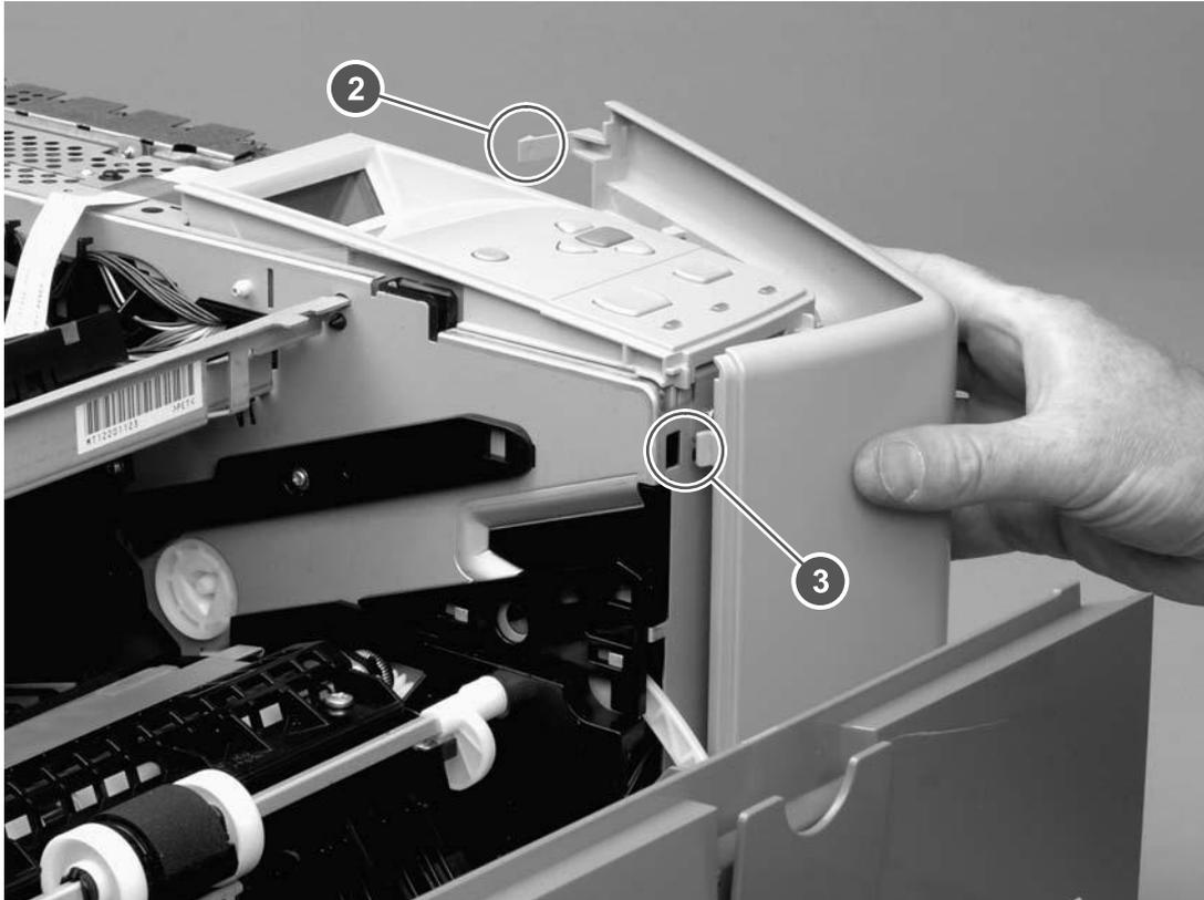
Figure 6-12 Removing the front, right cover (2 of 2)
