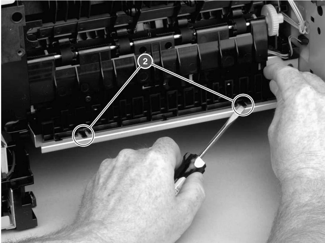
Figure 6-20 Removing the fuser (2 of 5)
