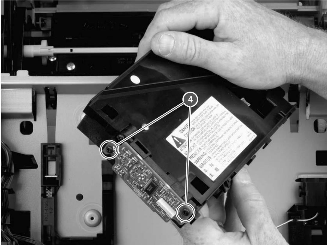
Figure 6-26 Removing the laser/scanner (3 of 3)
