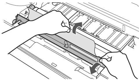
4. When the jammed media has been removed, gently flip down the registration plate. Reinstall the print cartridge and shut the top cover.
