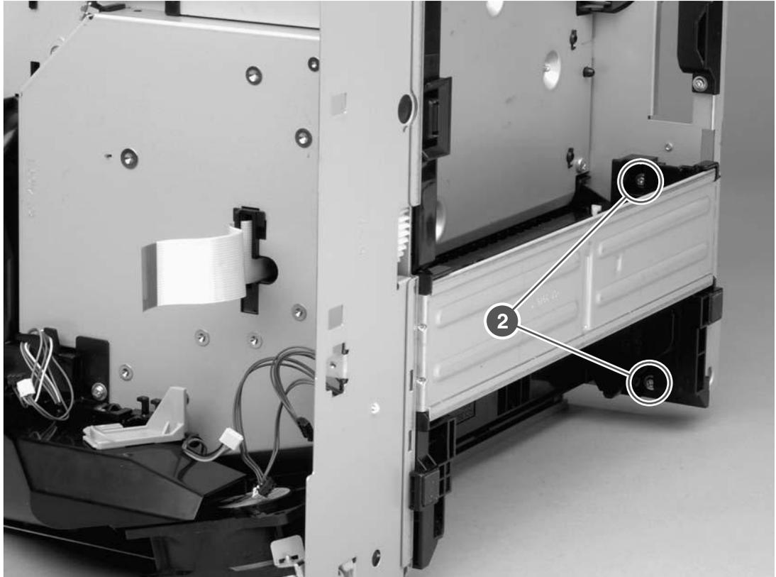
Figure 6-37 Removing the power supply (2 of 5)
