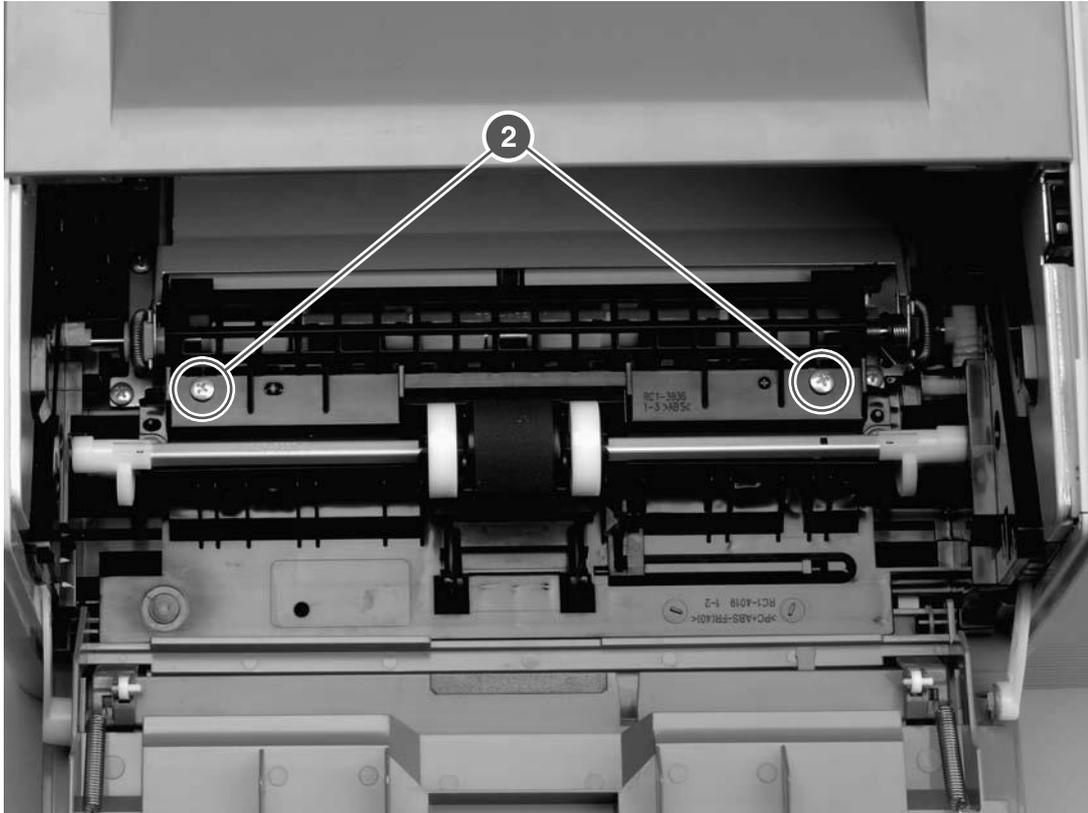
Figure 6-56 Removing the registration assembly (2 of 3)
