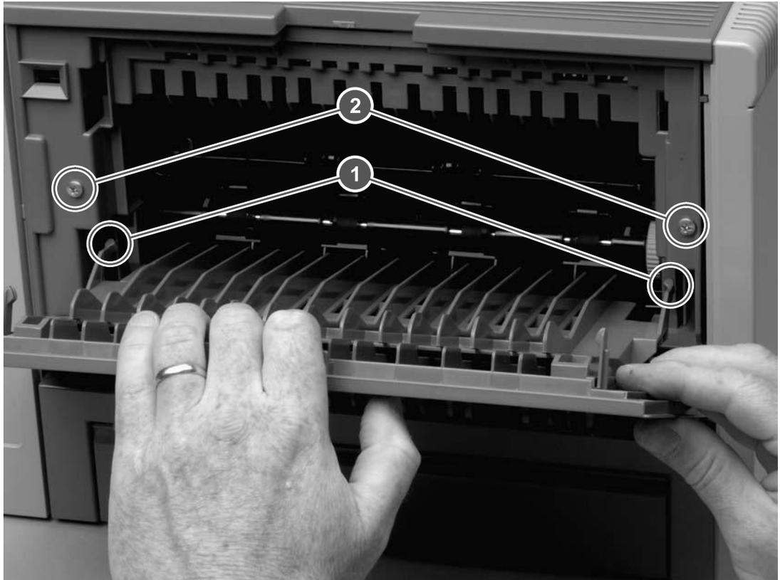
**Figure 6-3** Removing the back cover (1 of 3)
