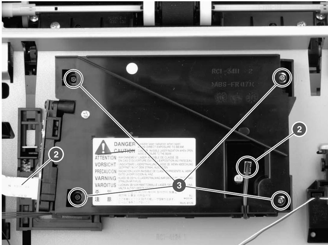
Figure 6-25 Removing the laser/scanner (2 of 3)
