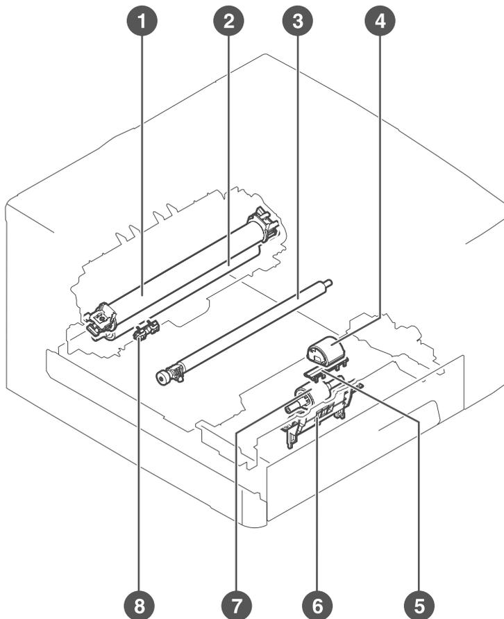
Figure 7-7 Main parts, HP LaserJet 2400 series
