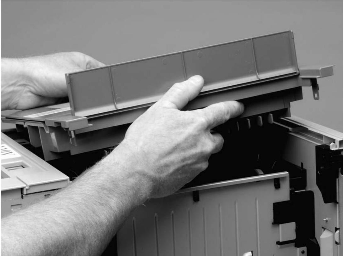
**Figure 6-5** Removing the back cover (3 of 3)
