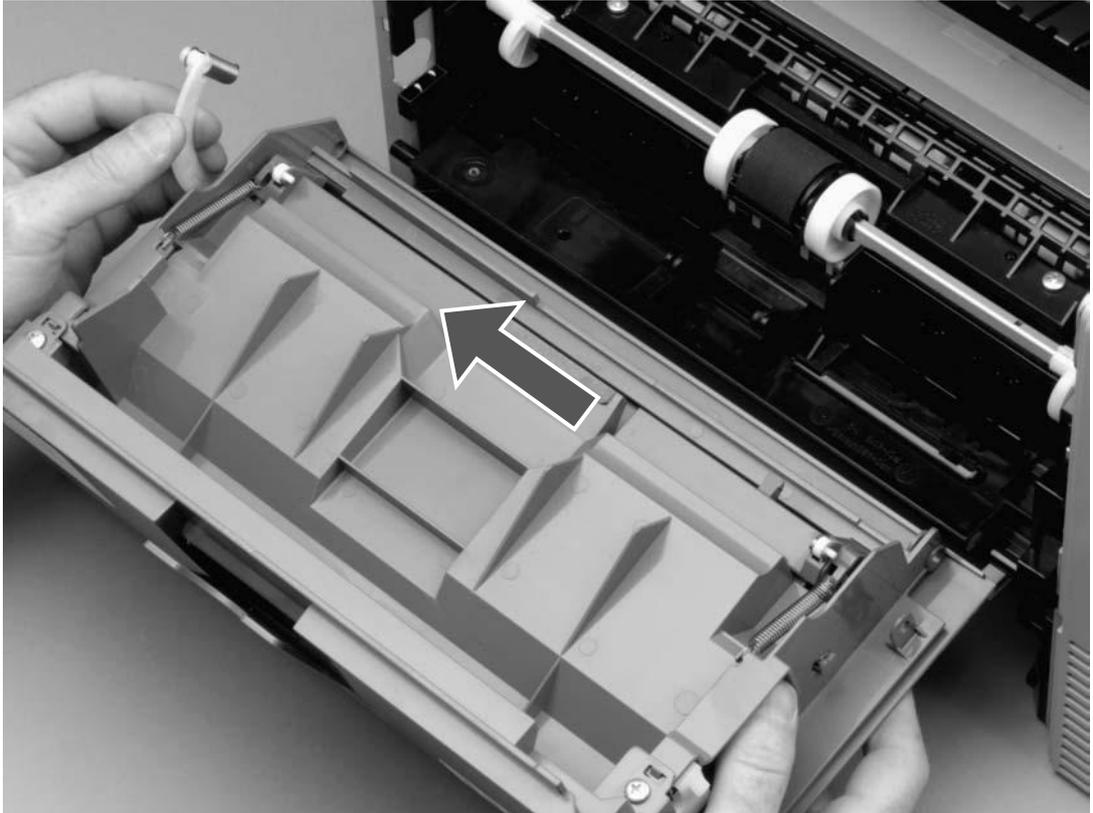
Figure 6-53 Removing the cartridge door (3 of 3)
