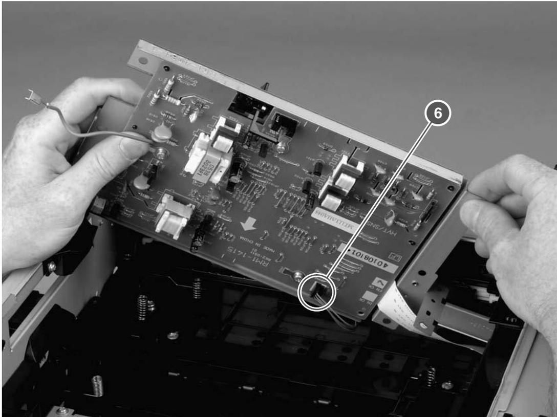
Figure 6-40 Removing the power supply (5 of 5)
