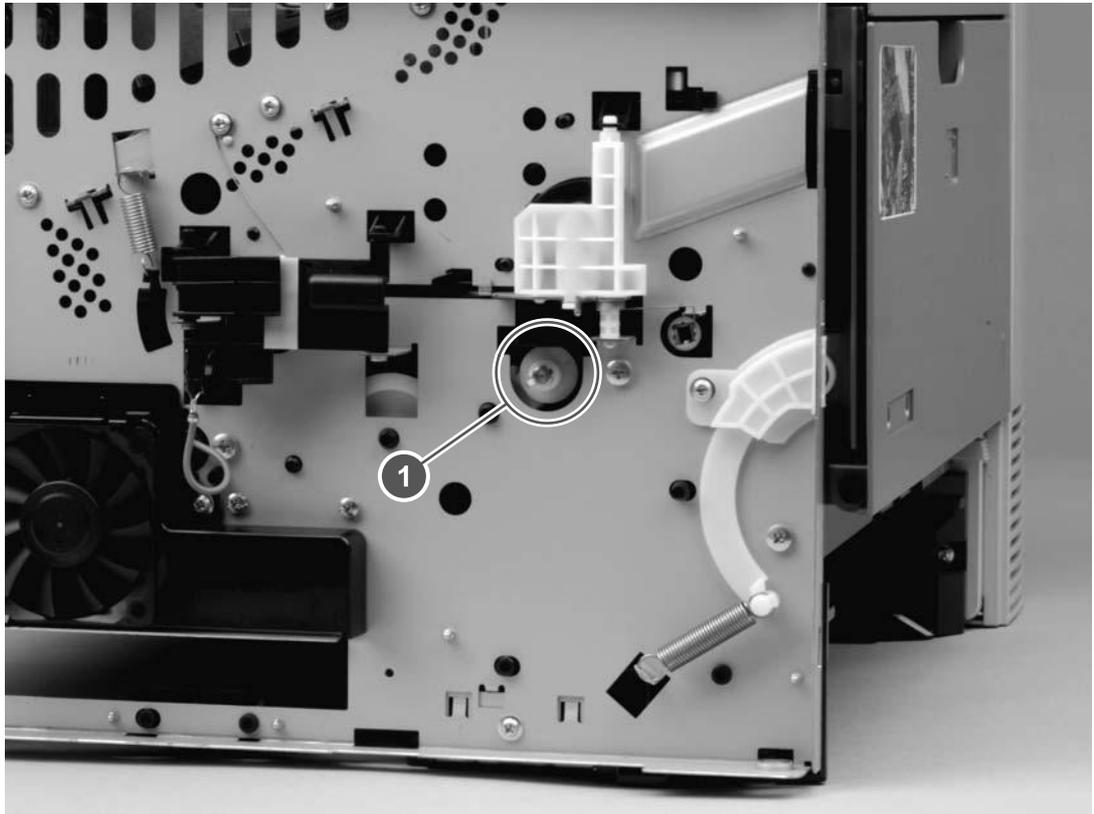
Figure 6-55 Removing the registration assembly (1 of 3)
