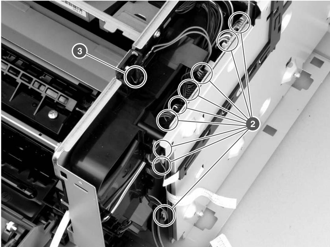
Figure 6-30 Removing the ECU (2 of 6)
