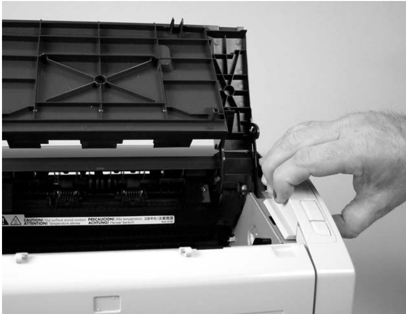
Figure 5-7 Remove the right-side cover (3 of 4)
