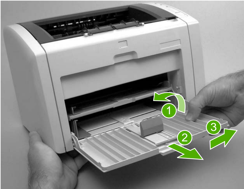
Figure 5-3 Remove the main input tray
