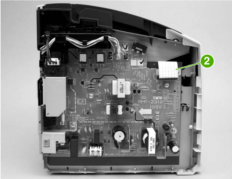
Figure 5-29 Remove the ECU assembly (2 of 6)
