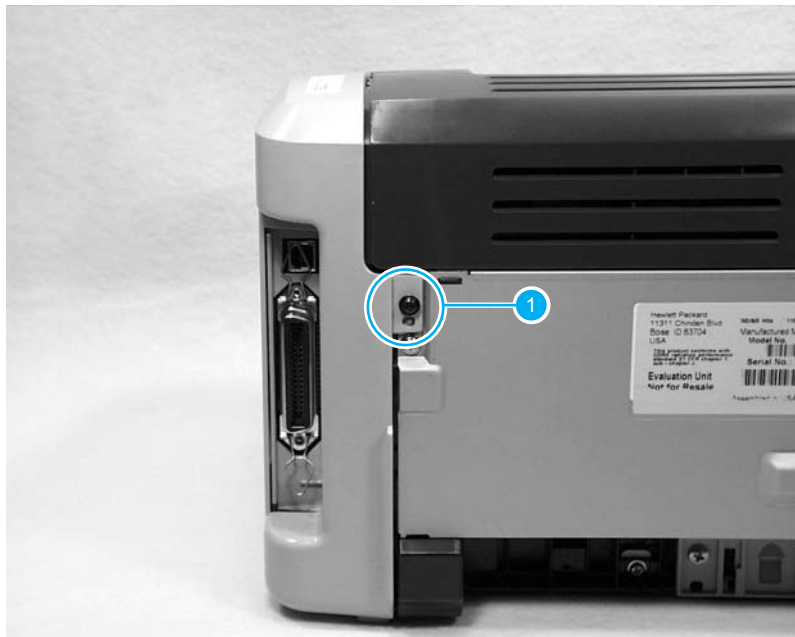
Figure 5-5. Removing the right side cover (2 of 5)
