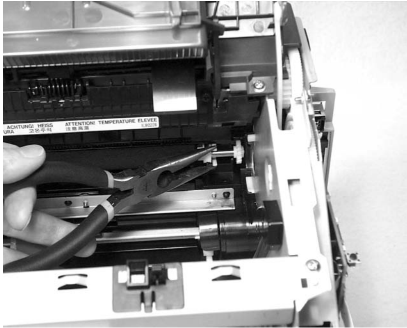
Figure 5-19. Removing the transfer roller (3 of 3)
