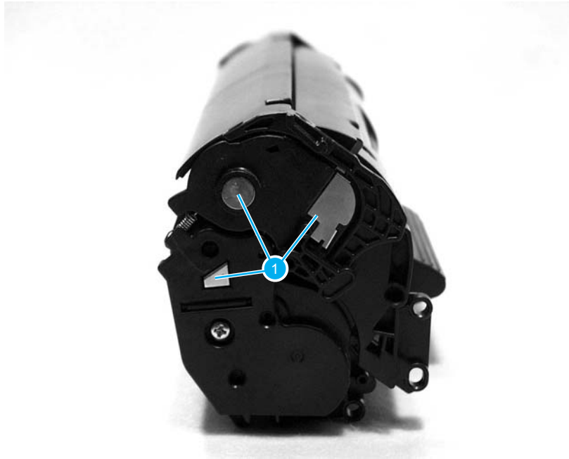
Figure 6-3. Print cartridge high-voltage contacts
